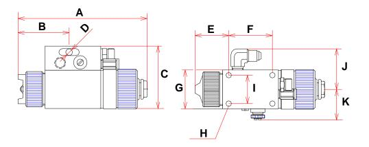
Fixing the gun onto its base : 4 screws M 6 x 50.
