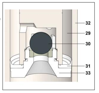
Apply a light coating of grease to the threading of exhaust valve (33) (grease, type A2). Screw the part in the piston lower part (29) (refer to greases in § Assembly instructions).
