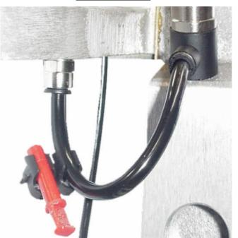
The motors mounted in our plant are cabled in **standard piloting.** The threshold of the motor starting is about 1.5 bar / 21.7 psi.
