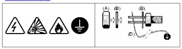
Loosen the lock nut (A), introduce between the washers (B) the end of an earth-wire (D) (minimum section: 1.5 mm2) into the hole of the terminal. Tighten the lock nut (A). Connect the other end of the wire to a real ground according to the local rules.
