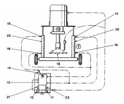
The motor is coupled to the hydraulic section piston. When the piston is raising and lowering the material is siphoned and dispensed simultaneously.
