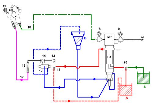
This pump measures and mixes 2 components A and B to a single defined volume proportion (see data sheet of the product).
