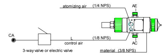
The A28 spray gun works by pneumatic command. To make it work, it simply requires either an electronic valve or a three-way pneumatic valve. The electronic valve must be placed as close as possible to the gun (L  $\sim$  2 m / 6.6 ft).
