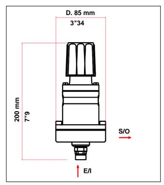
The LP fluid regulator with integrated pilot enables to allow a constant pressure.
