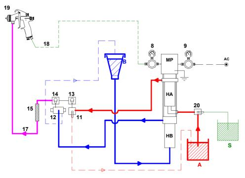
This pump measures and mixes 2 components A and B to a single defined volume proportion (see data sheet of the product).
