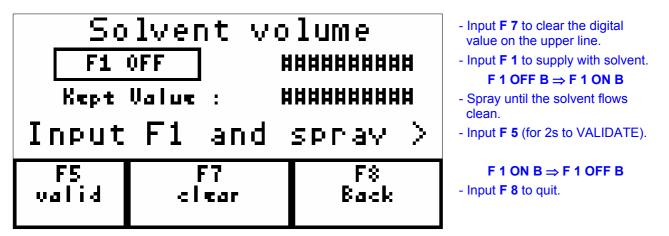
That parameter is used for the flushing of production.
