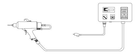
Power supply to control unit: 220 V. Power supply to the spray gun: 24 V.
