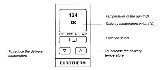
The display at the top of the unit shows the temperature of the gun. If this temperature is less than the required delivery temperature, the regulator sends a signal to heat up. This is accompanies by a warning light (OP 1). Once the system is back up to temperature, this light goes out.
